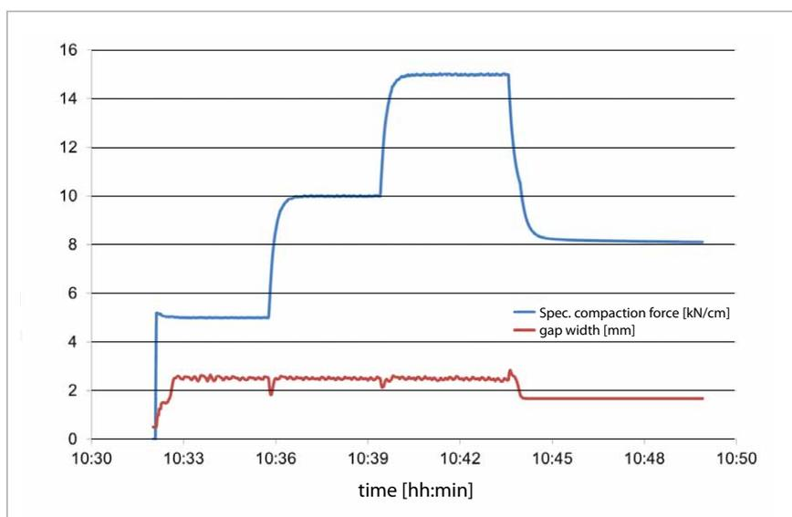
Figure 1: Gap width over time at increasing compaction force values
