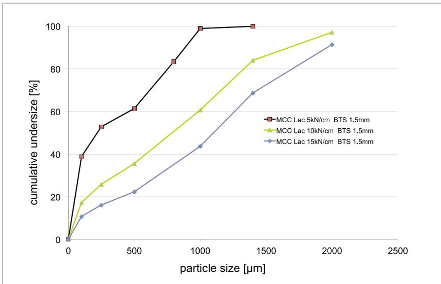
Figure 2: Compaction force impact on granule particle size
